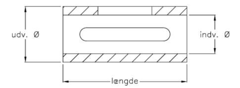
Description = 14/24Internal diameter = 14Length = 40Outer diameter = 24
